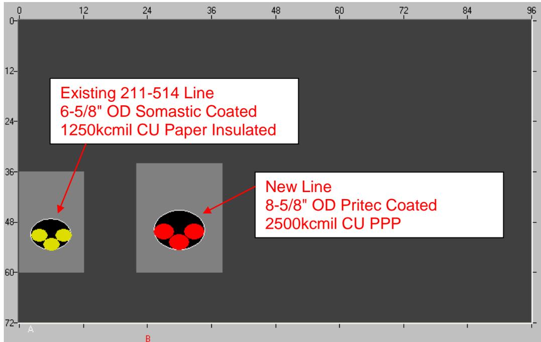
**Figure 3.1 Schematic of the Configuration for the Existing and Proposed Lines.** The x-y coordinate system origin is at the street surface in the upper left corner of the figure. The conductor locations shown are illustrative, and the figure is not to scale. Typical depth variations created during installation would have a small effect on the calculated magnetic field values.
